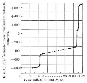
Fig. 2.—Graph representing potentiometric titration of 30 cc. of reduced uranyl solution with ceric sulfate (0.1043 N). The inflection at the left corresponds to the end of the oxidation of  $U^{\rm III}$  to  $U^{\rm IV}$ ; the next to oxidation of  $U^{\rm IV}$  to  $U^{\rm VI}$  and the last to Fe<sup>II</sup> to Fe<sup>III</sup>.
