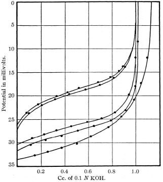
Fig. 2.—Titration curves with the quinhydrone electrode in 60% butyl carbitol. 0.005~M acids titrated with 0.1~M KOH. In order, from the top, acetic, benzoic, o-nitrobenzoic, chloroacetic, dichloroacetic,
