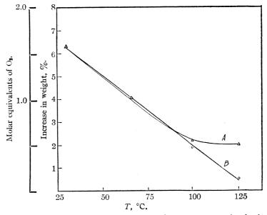
Fig. 4.—Maximum oxygen absorbed at various temperatures by lead rosinate: A, actual O<sub>2</sub> absorbed; B, apparent O<sub>2</sub> absorbed.
