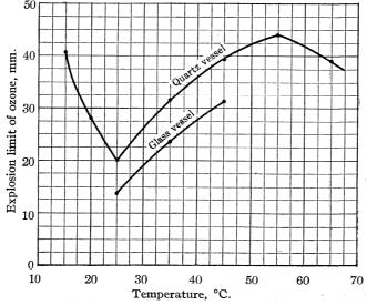
Fig. 4.—Effect of temperature on the explosion limit.
