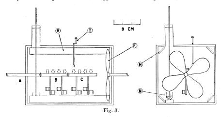
The air-bath was very heavily lagged with transite and magnesia board. It was provided with a mica window, kept covered except when it was desired to inspect the tubes. The top of the bath was provided with removable sections to allow inserting the brackets with care and also breaking the capillaries.
