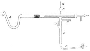
Fig. 1.—Apparatus for the preparation of zirconium tribromide.
