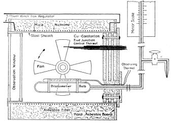
Fig. 3.—The thermostat as used with the dilatometer.
