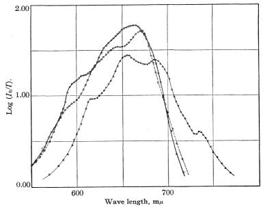
Fig. 4.—The absorption spectra of cobalt quinolinium halogen complexes  $((QH)_2CoX_4)$  in absolute ethyl alcohol: X = Cl,  $\longrightarrow$ ; Br, -----; and I,  $\longrightarrow$ . The cobalt pyridinium complexes gave identical curves.
