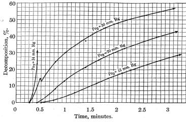
Fig. 1.—Typical curves showing decomposition of ozone: T, 35°; Br<sub>2</sub> pressure, 5 mm.
