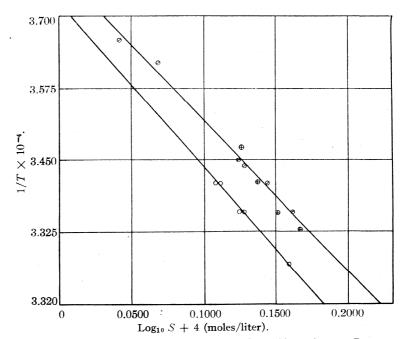
Fig. 4.—Solubility of lead sulfate in water.  $\ominus$ , Kohlrausch;  $\bigcirc$ , Böttger;  $\ominus$ , Huybrechts and de Langeron.
