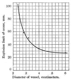
Fig. 5.—Relation between explosion limit at 25° and diameter of vessel.
