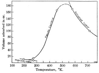
Fig. 1.—Adsorption isobar of hydrogen on manganous—chromic oxide at  $P=165~\mathrm{mm}$ .
