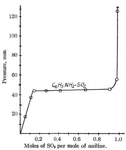
Fig. 1.—Pressure-composition diagram, aniline + SO<sub>2</sub> at 25°.
