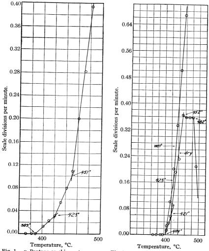
Fig. 1.—n-Pentane cracking rate curve: 1 Scale div. = 0.09 cc. at 40°.
