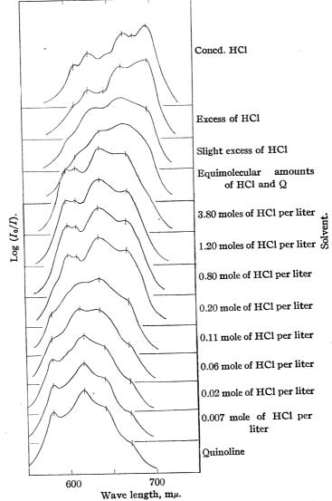
Fig. 8.—The change from the "Py-Q" system, through the "intermediate" system to the "HX" system, caused by the addition of HCl to a solution of CoCl<sub>2</sub> in quinoline. (The curves in this figure are only a few of the some fifty curves, observed at various Q-HCl concentrations. They have been chosen to show characteristic stages or transition points in the change of the absorption systems. The concentration of CoCl<sub>2</sub> in all solutions was approximately 0.0043 mole per liter.)
