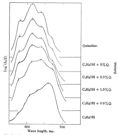
Fig. 7.—The change from the alcohol absorption to the "Py-Q" system of absorption caused by the addition of quinoline to a solution of CoCl<sub>2</sub> in ethyl alcohol.
