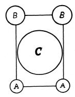
Fig. 1a.—If the substitution of (C) increases the absolute dimension of the cell from  $4 \times 10$  to  $8 \times 12$ , the axial ratio changes from 1:2.5 to 1:1.5.
