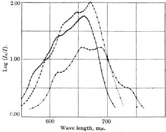
Fig. 5.—The absorption spectra of cobaltous halides in ethyl alcohol: Cl, ———; Br, -----; and I, ———.
