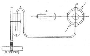
Fig. 1.—Apparatus for measuring magnetic susceptibilities.
