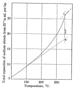
Fig. 4.—The expansion curve of sodium nitrate from 100° upward. The open and the black circles differentiate between ascending and descending sequence of constant temperatures. The distance BC is a measure of the anomalous expansion. Note the gradual character of the curve.
