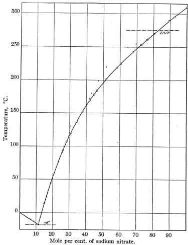
Fig. 7.—The solubility of sodium nitrate in water. The larger open circles by Kracek. The small black circles above  $100^{\circ}$  are by Étard. Results below  $100^{\circ}$  by Berkeley and others.
