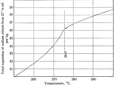
Fig. 5.—The expansion curve of sodium nitrate near 275°. Note the reproducibility of the curve as indicated by the open and black circles which differentiate between rising and falling sequence of constant temperatures, and the absence of a sharp break at 275°.
