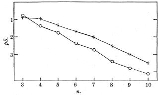
Fig. 1.—Solubility of ethyl esters of monocarbonic acids ( $\bigcirc$ ) and of dicarbonic acids (+) in water at 20°: n, number of carbon atoms;  $pS_n - \log_{10}$  of normality of saturated solution.
