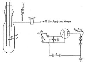
Fig. 1.—Tube with electrical connections.
