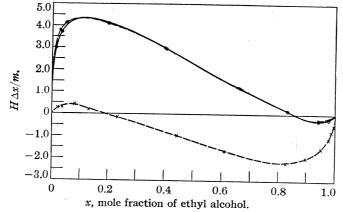
Fig. 2.—Silica (experimental), ————; carbon (experimental),  $\times$  ———; 8.8105 (x)<sup>0.227</sup> (1 — x) — 4.664 (1 — x)<sup>0.615</sup> (x), O ———. Adsorption of ethyl alcohol from benzene.
