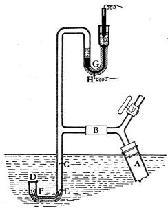
Fig. 1.—Diagrammatic view of the bubble counter.
