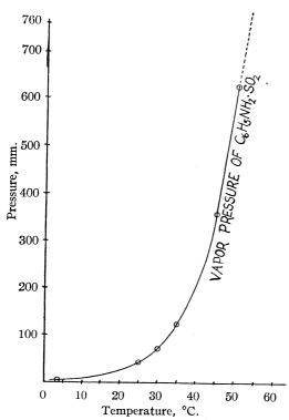
Fig. 2.—Vapor pressure of C<sub>6</sub>H<sub>5</sub>NH<sub>2</sub>·SO<sub>2</sub> at varying temperatures.
