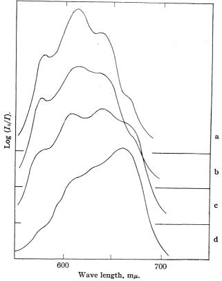
Fig. 3.—(a) The absorption spectra of cobaltous chloride—pyridine complex (CoPy<sub>2</sub>Cl<sub>2</sub>) in CHCl<sub>3</sub>; (b) CoPy<sub>2</sub>Cl<sub>2</sub> in CHCl<sub>3</sub> + C<sub>2</sub>H<sub>5</sub>OH; (c) CoPy<sub>2</sub>Cl<sub>2</sub> in C<sub>2</sub>H<sub>5</sub>OH; (d) (PyH)<sub>2</sub>CoCl<sub>4</sub> (cobaltous pyridinium chloride) in C<sub>2</sub>H<sub>5</sub>OH.
