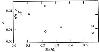
Fig. 4.—Variation of k with change in  $(H_2O_2)$ .  $(H^+) = 0.0677$ ;  $(IO_3^-) = 0.0142$ .
