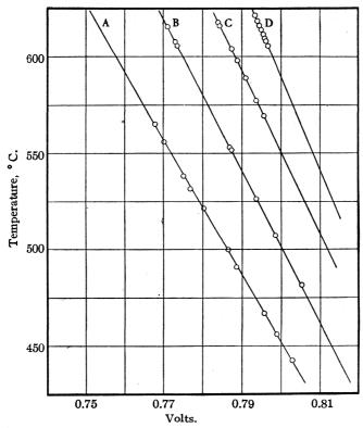
Fig. 1.—Temperature, e. m. f. and composition relations of the cells Ag/AgBr, NaBr/Br<sub>2</sub>. Mole fraction of silver bromide in A is 1.000, B is 0.7486, C is 0.6045 and D is 0.5130.
