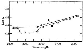
Fig. 2.—Log extinction coefficient—wave length curves for: A, chlorophyll a; B,  $\times\times\times$ , allomerized chlorophyll a;  $\bigcirc\bigcirc\bigcirc$ , dehydrochlorophyll a.
