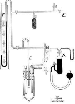
Fig. 1.—Apparatus for finding melting points, boiling points and vapor pressures of krypton and venon.
