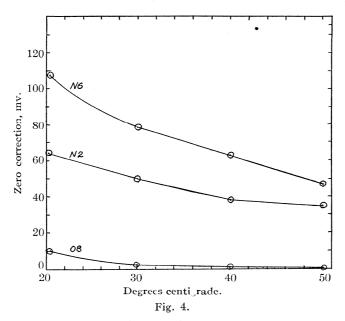
used. Curves showing the relationship between zero correction and temperature are shown in Fig. 4, these measurements being made with the electrometer. In Fig. 4, 08 is a thin electrode; N2 and N6 are thicker electrodes. Additional measurements on a good electrode in a buffer
