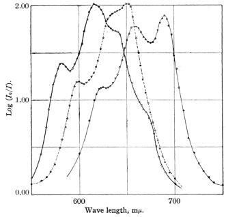
Fig. 2.—The absorption spectra of cobaltous halides in quinoline: ——, CoCl<sub>2</sub>; -----, CoBr<sub>2</sub>; ——, CoI<sub>2</sub>. (Identical or nearly identical curves were obtained from cobalt quinolinium halides in quinoline and cobalt halides and cobalt pyridinium halides in pyridine.)
