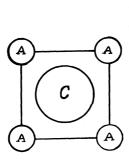
Fig. 1.—If the substitution of (C) increases the absolute dimension of the cell from  $5 \times 5$  to  $10 \times 10$ , the axial ratio is not changed.
