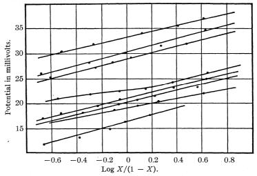
Fig. 1.—Titration curves with the antimony electrode in 60% butyl carbitol. 0.05~M acids titrated with 1.0~M KOH. In order, from the top, stearic, benzoic, acetic, formic, salicylic, chloroacetic, malonic, dichloroacetic (stearic acid at 0.005~M, titrated with 0.1~M KOH).
