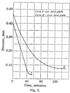
line is identical to similar time—pressure curves obtained in the glow discharge in that the rate is independent of the pressure over a wide range. The rapid dropping of the rate to zero at some minimum pressure characteristic of the discharge tube is common also to both types of arcs. It will be noted that the rate remains constant to 0.04 mm. pressure while no synthesis could ever be detected under 0.02 mm. with a plate diameter of 1 cm. or less.
