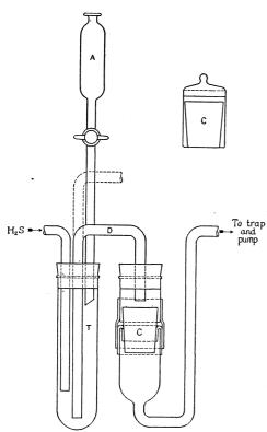
Fig. 1.—Apparatus for the preparation of amine hydrosulfides.
