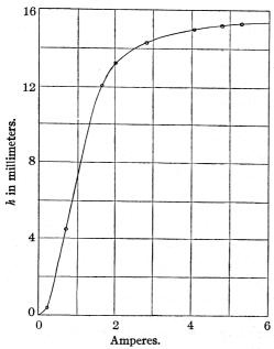
Fig. 2.—Variation of rise of liquid in magnetic concentrated solutions h was field with current through magnet.
