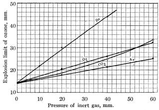
Fig. 6.—Effect of inert gases on the explosion limit at 25° (5 mm. of bromine).
